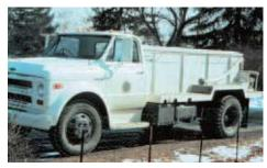
Distribution vehicle, equipped with a fourcompartment tank, pony motor and pump, was used from mid-1950 to mid-1970. holding trout. In fact, fish-distribution problems these days are rare.
