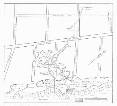
FIG. 3. Generalized sketch map of the vicinity of the Schuyler or Arlington copper mine. There is no present surface indication of the old Victoria shaft at street level, and considerable areas over the large chambers near Morton Place are partially caved. The reduction plant of the Arlington Copper Company is mostly in ruins, save the building on the meadow floor, which is currently occupied. Location of the underground workings is based upon a published map by O. Ivan Lee.
