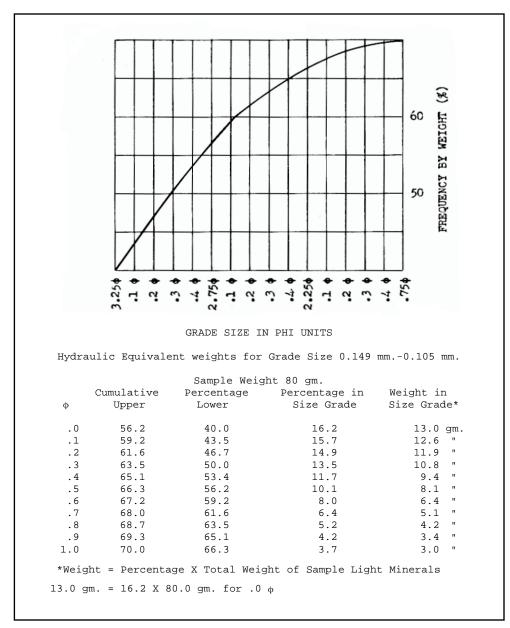
Figure 6 Computation of Hydraulic Equivalent Weights
