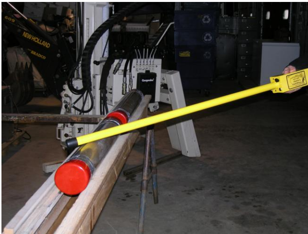
Figure 5. Geophysical prove-out using Schonstedt GA 52CX™ detector.
