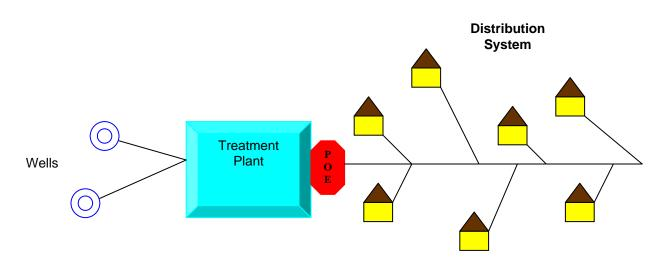
Figure 2: POE and Distribution System of a Community Water System
