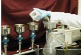
2: Filter water sample onto membrane filter
