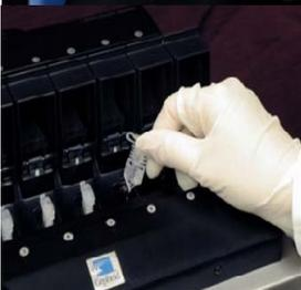
7: Place reaction tube into thermal cycler
