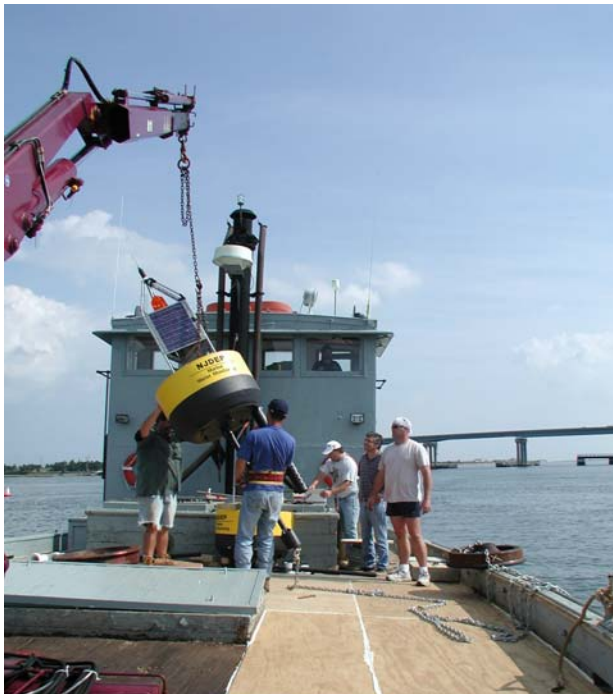
Deployment of buoy for continuous monitoring of coastal water quality parameters
