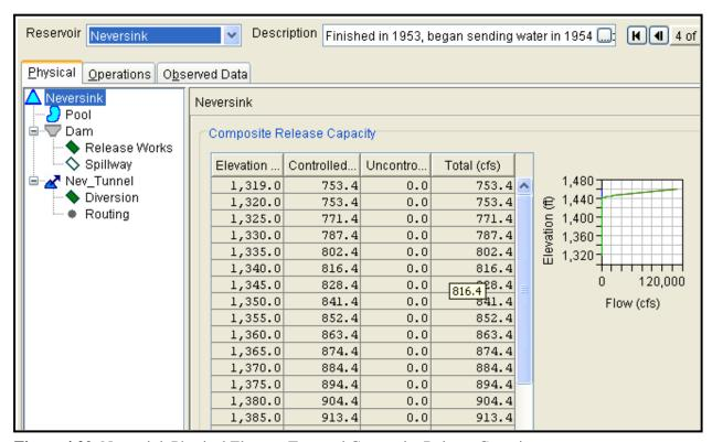
Figure 4.20 Neversink Physical Element Tree and Composite Release Capacity
