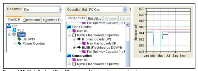
Figure 4.32 Rio's Pool and Dam Elements and its operating zones & rules
