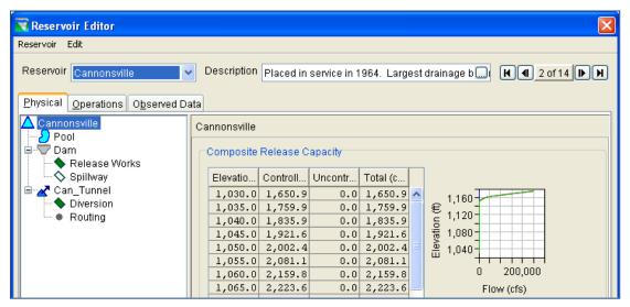
Figure 4.9 Cannonsville – Physical Element Tree and Composite Outlet Capacity Table
