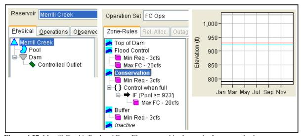
Figure 4.37 Merrill Creek's Pool and Dam Elements and its "operating" zones and rules
