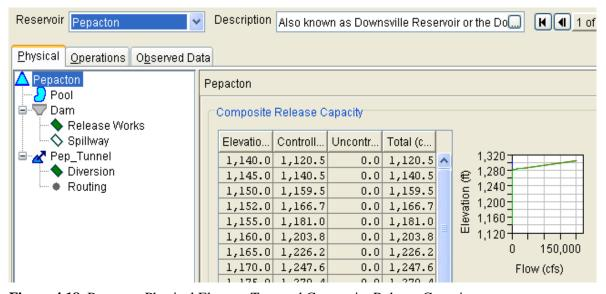
Figure 4.18 Pepacton Physical Element Tree and Composite Release Capacity
