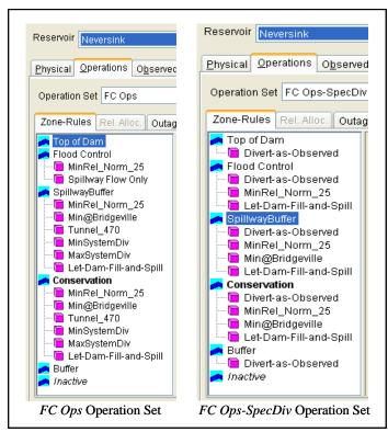
The operations at Neversink were described with the operations at Cannonsville. Table 4.15 and Table 4.16 summarize these operations. An important difference at Neversink is that in the *FC Ops* operation set, no Ifblock was used to correlate the suspension of the diversion to conditions at the other reservoirs in the system. In the model, the suspension was triggered by pool elevation and is represented by the *Spillway Flow Only* rule in the *Maximum Pool* zone.
