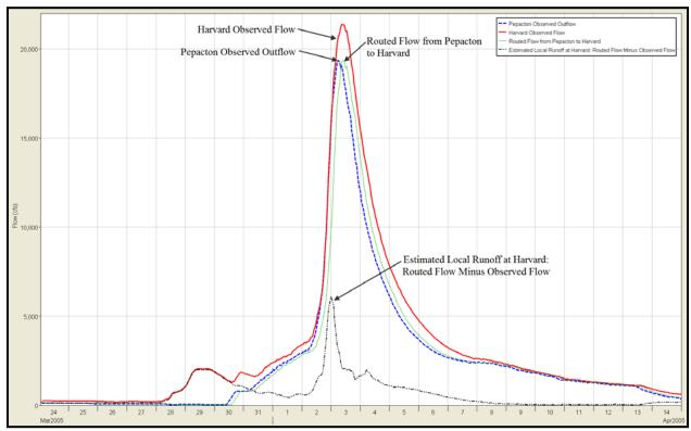
Figure 5.1 Example Showing how Local Runoff at Harvard was Estimated for the 2005 Event
