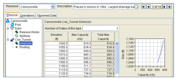
Figure 4.15 Cannonsville's Diverted Outlet – Can\_Tunnel
