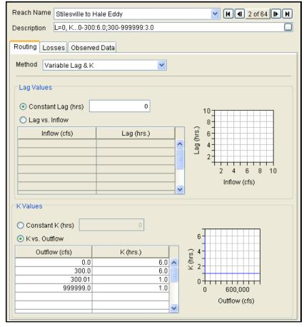
Figure 4.6 Stilesville to Hale Eddy, Lag & K Routing – Variable K
