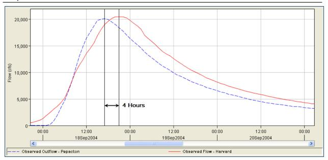
Figure 4.4 Observed Releases from Pepacton Reservoir and Observed Discharge at Harvard
