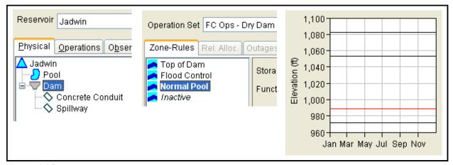
Figure 4.25 Jadwin's Pool and Dam Elements and its "operating" zones
