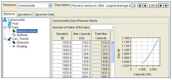
Figure 4.12 Cannonsville – Release Works
