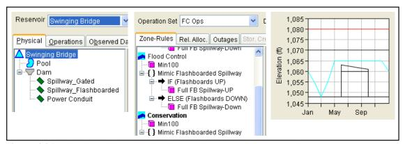
Figure 4.31 Swinging Bridge's Pool and Dam Elements and its "operating" zones
