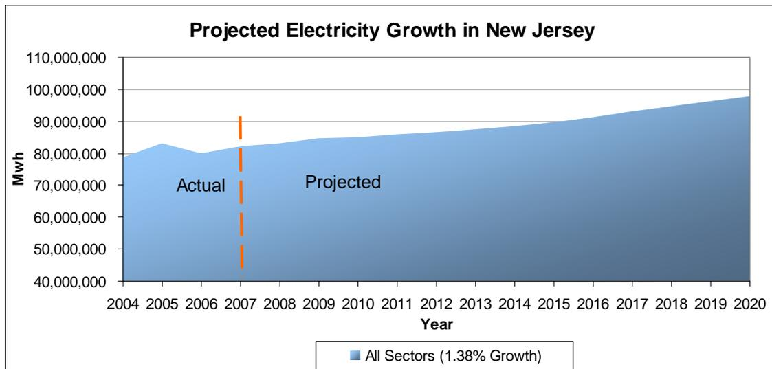
**Figure 1: Projected Growth in Electricity Consumption.** If New Jersey does not act to change its energy use, demand is conservatively expected to grow 1.38% per year, leading to an increase in use of 15,800 GWh between 2007 and 2020.
