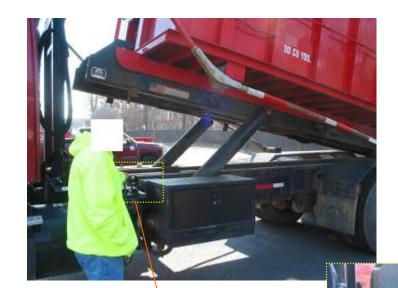
Left knob controls the bed hoist (up/down)
