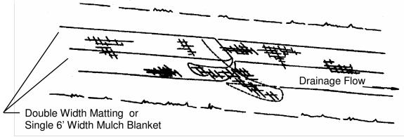
Overlap: Bury upper end of lower strip as per above detail. Overlap end of top strip 6" (150 mm) and staple either side of joint.
