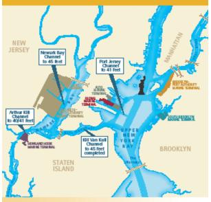
Deepening of channels at several critical access points allows larger containerships with more cost-efficient loads to enter the harbor.
