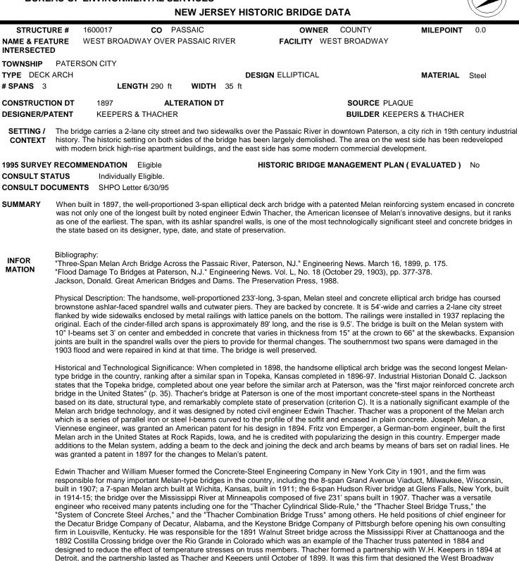
The Thacher & Keepers-designed Melan-type arch bridge is one of two in the state designed by Edwin Thacher. The other is located in Branch Brook Park in Newark (Essex County) (0700101). It was designed by the Concrete-Steel Engineering Company in 1905. Both are technologically and historically important as examples of the experimentation associated with the introduction of concrete and steel arch bridges in this country.
