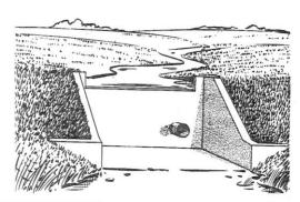
I. <u>Grade Stabilization Structure</u> – Water Control Structure(s)
