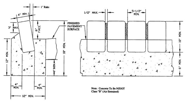
VERTICAL GRANITE BLOCK CURB (With Concrete Gutter)
