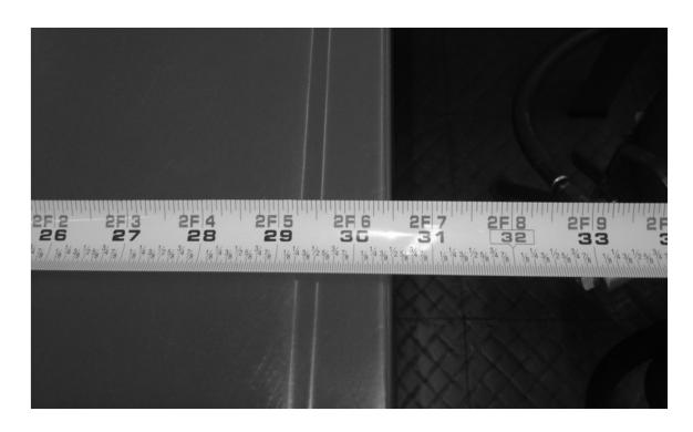
DO NOT **MEASURE** WITH THE LID DOWN (30.5" with lid down = **INCORRECT** measurement)
