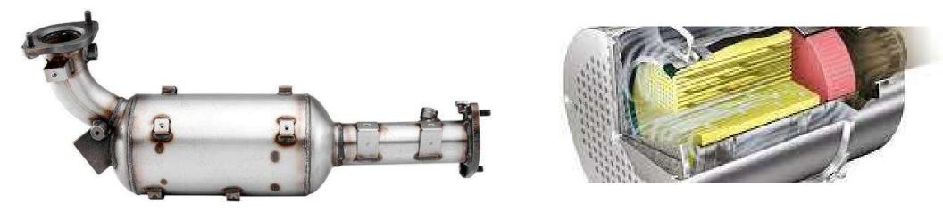
A diesel particulate filter, or DPF, is an exhaust aftertreatment device that traps particulate matter such as soot and ash. A DPF typically uses a substrate made of a ceramic material that is formed into a honeycomb structure.
