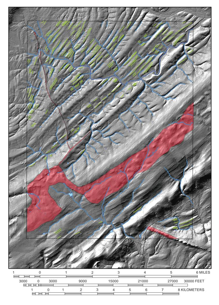
Figure 1. LIDAR (Light Detection And Ranging) map of the Hopewell quadrangle showing the correlation of igneous units and strike of ridge lines (green) with topography.
