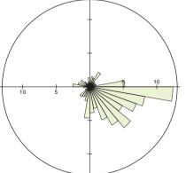
Sector angle = 10° Maximum = 13% Dip azimuth of joints in Passaic Fm
