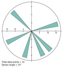
Maximum = 18% Dip azimuth of joints in Stockton Fm
