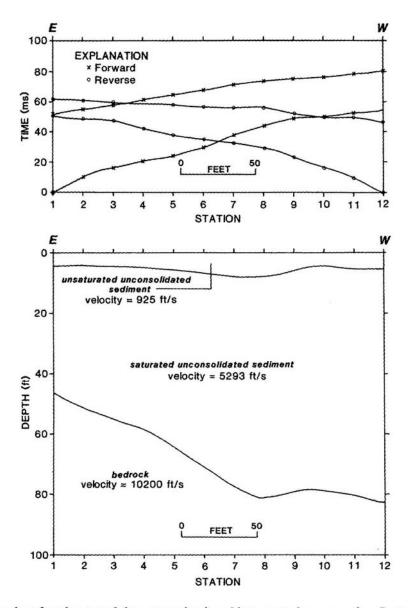
Figure 6. Seismic refraction travel time curve (top) and interpreted cross section (bottom) for line 2.
