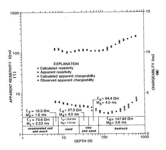
Figure 7. Electrical resistivity-IP sounding EHVES-2 with interpretation.
