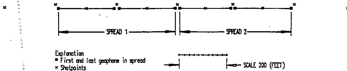
Figure 5. Seismic refraction field array showing shotpoint and geophone locations.
