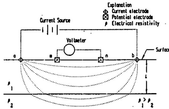
Figure 2b) Schlumberger electrical resistivity array geometry showing lines of current flow between electrodes for a two layer case (from Dobrin, 1976, fig. 17-7, p. 578).
