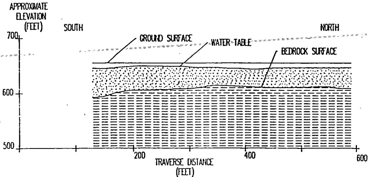
Figure 6. Interpreted seismic profile, traverse CD 5, Cooley Brook site.
