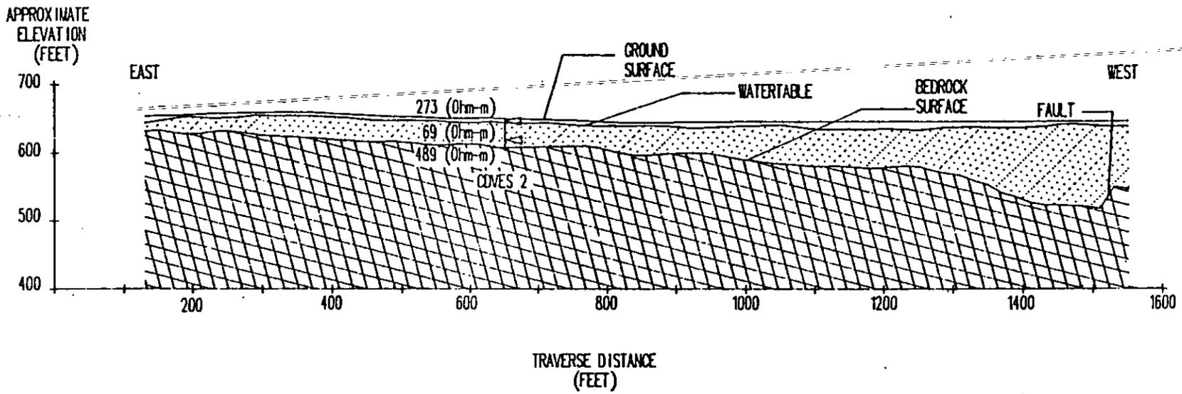
Figure 11. Interpreted seismic profile CD 7, Wallisch Property site, showing the location of resistivity sounding CDVES 2.
