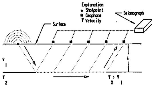
Figure 2 a) Seismic refraction energy raypath of a two layer case (modified from Dietrich, 1978, AGI data sheet 59.1).
