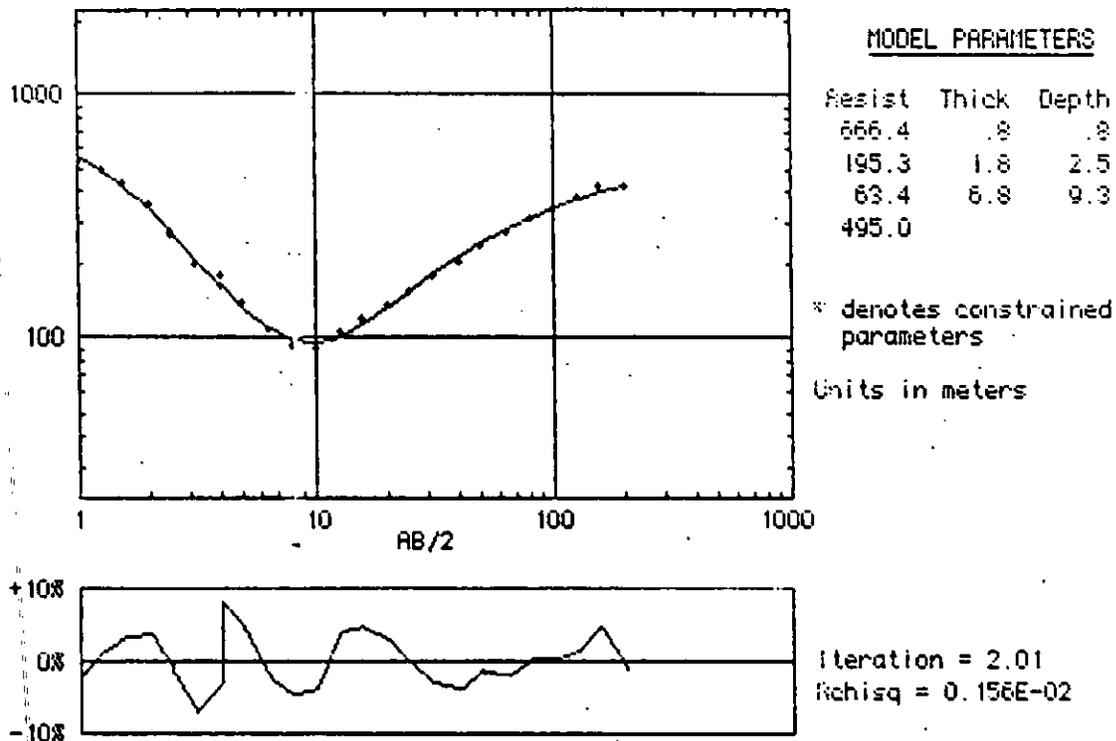
Figure 16. Resistivity modeling plot for sounding CDVES 2, Wallisch Property site.
