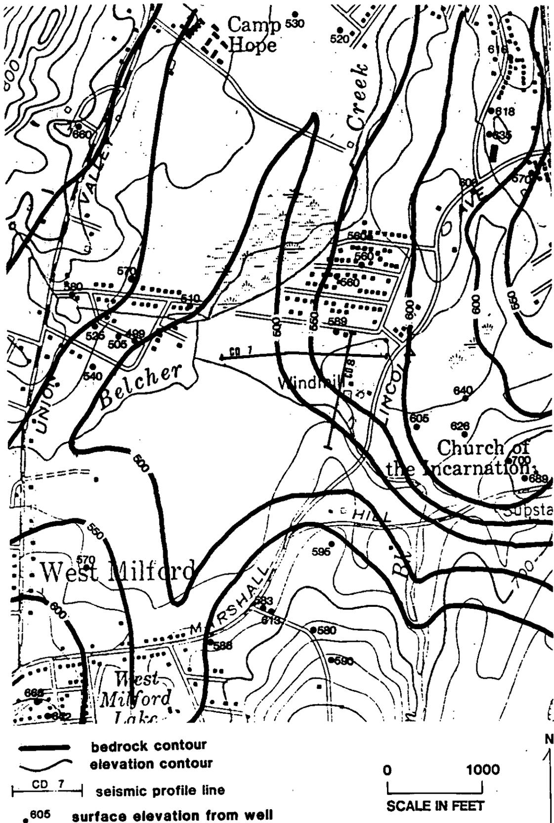
Figure 13. Bedrock contour map of the Wallisch Property site (modified from Stanford, unpub.).
