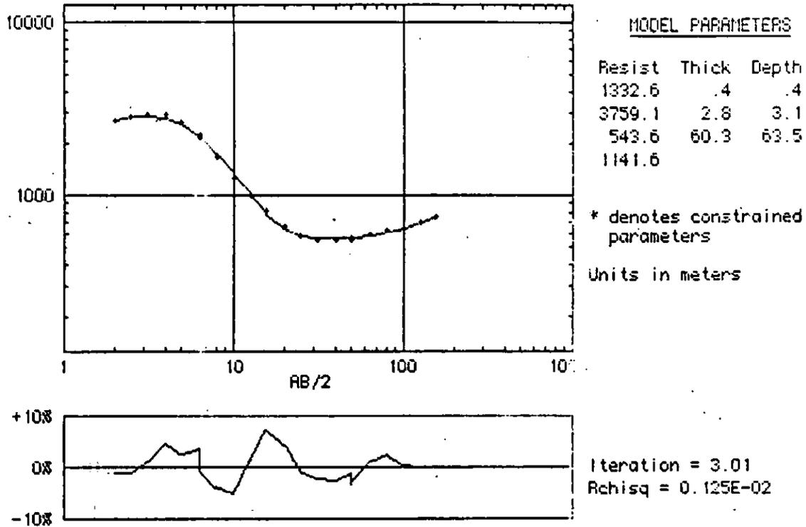
Figure 15a. Resistivity modeling plot for sounding CDVES 3, Cooley Brook site.
