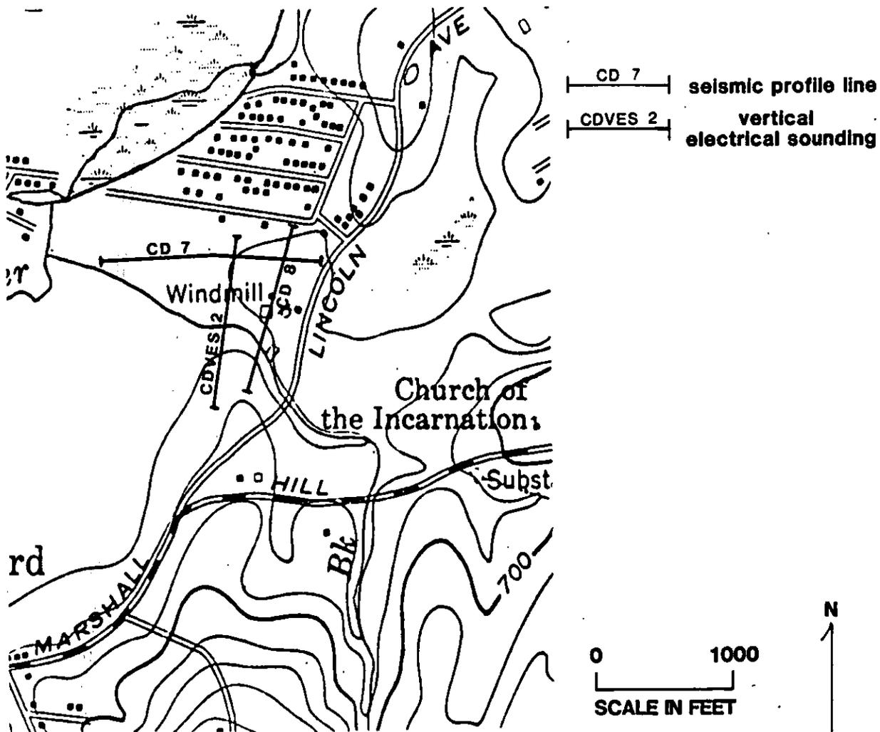
Figure 4. Geophysical survey locations at the Wallisch Property site.
