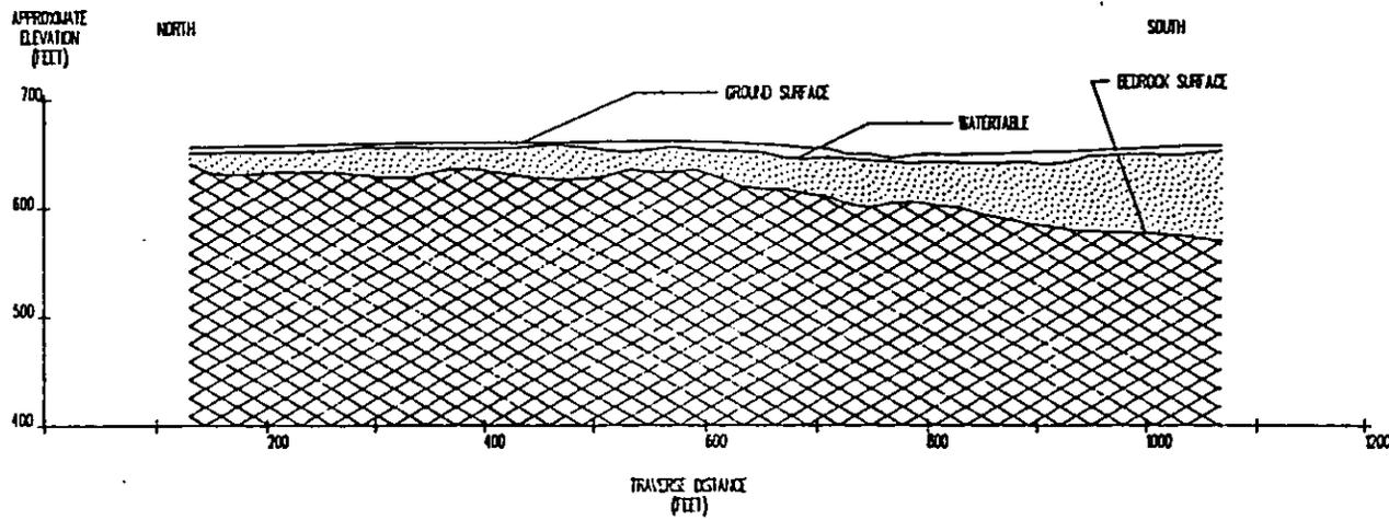
Figure 12. Interpreted seismic profile CD 8 at Wallisch Property site.
