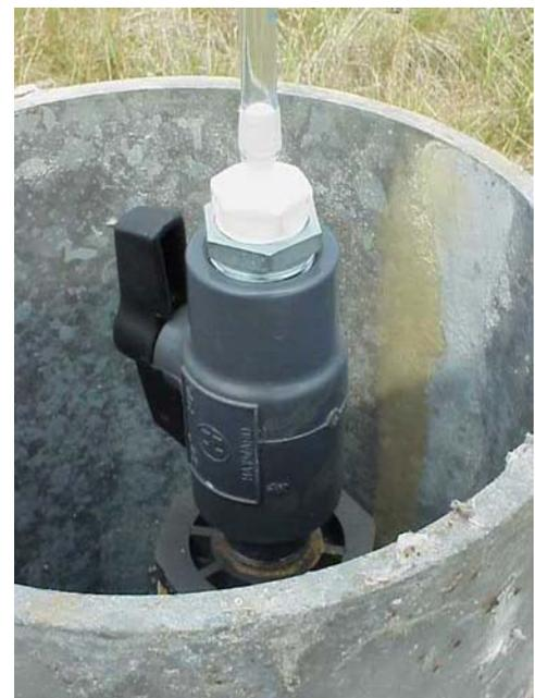
Figure 9.11 Ball Valve for Soil Gas Well, Photographed by C. Van Sciver
