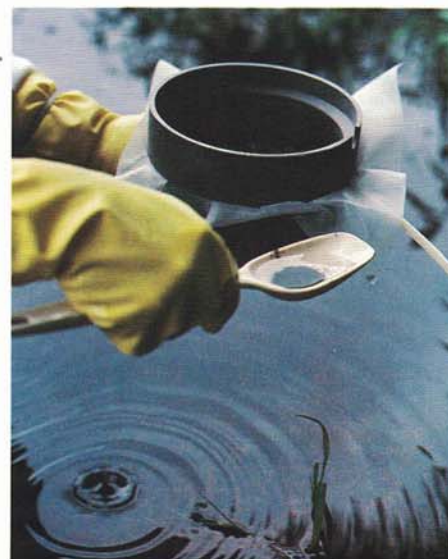
Sediment is spooned from the river bed, then placed in a sieve which screens out smaller particles for analysis.
