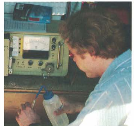
Todd Kratzer, DRBC water resources engineer, at work at a riverbank fluorometer, used to measure dye concentrations. (Photo by Chris Roberts)
