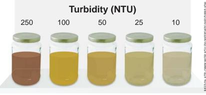
Turbidity, the amount of suspended material in water, is measured in nephelometric turbidity units (NTUs).
