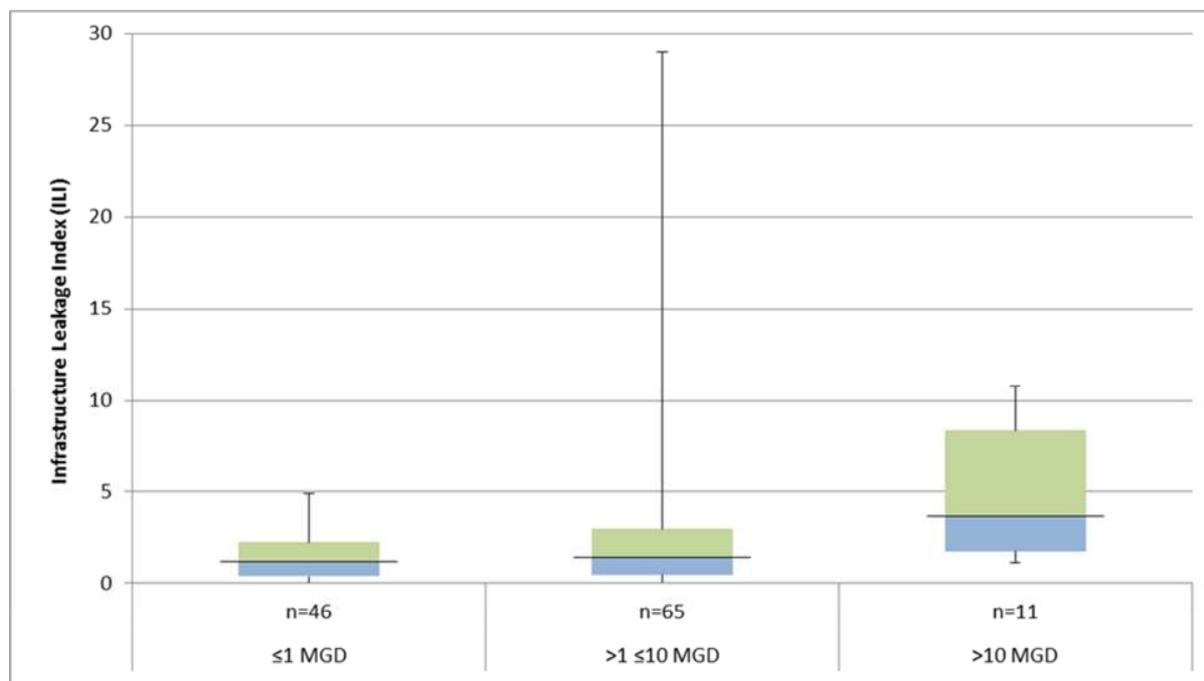
**Figure 11. Infrastructure Leakage Index (n = 122).** *Note that this performance indicator is not calculated for small or low pressure systems.*
