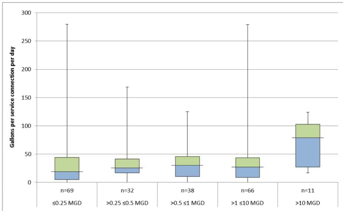
**Figure 10. Real Losses (Gallons per Service Connection per day), by System Size (n = 217). Note that this performance indicator is not calculated for systems with a low average service connection density (less than 32 connections per mile).**
