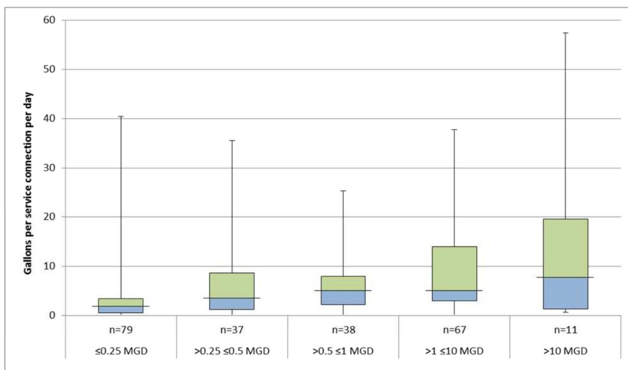
**Figure 9. Apparent Losses (Gallons per Service Connection per Day) by System Size (n = 232).**
