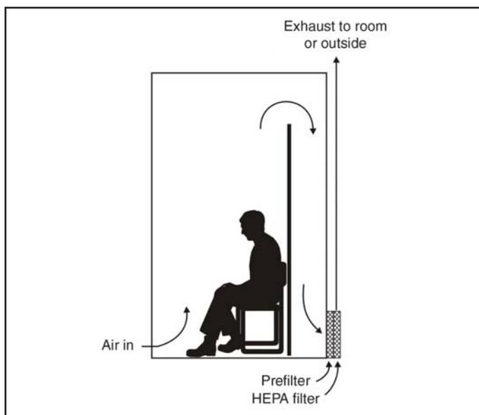
contained airflow and recirculation system (see Environmental Controls; Figure 2).
