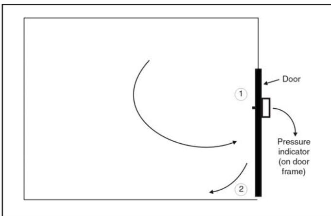
\* Airflow pressure at location 1 might differ from that at location 2. Measure pressure at location 2 for correct indication of negative pressure.
