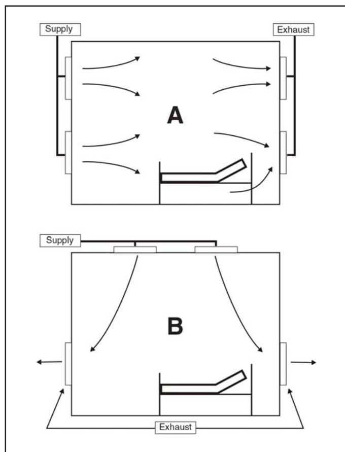
\* Short-circuiting is the passage of air directly from the air supply to the exhaust.
