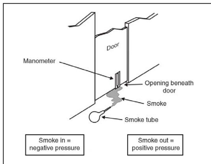
tive pressure. These simple and inexpensive devices are placed directly in the door and can be useful in identifying a pressure differential problem.
