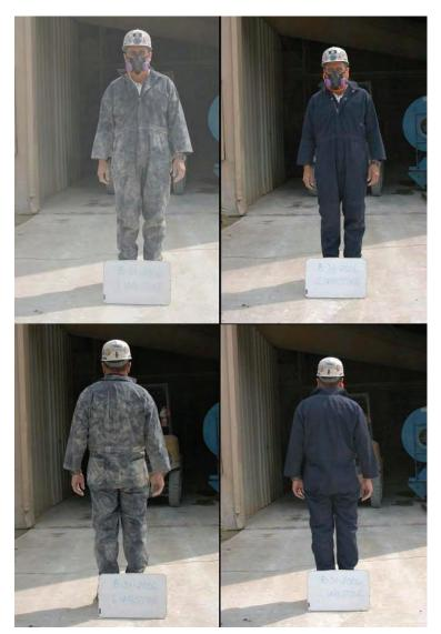
Figure 4-17. Test subject before and after using the clothes cleaning booth.
