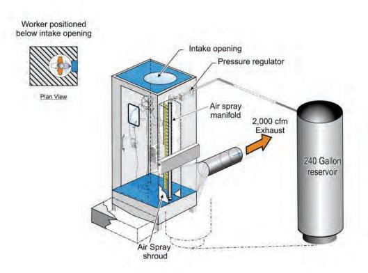
Figure 4-16. Clothes cleaning system design.
