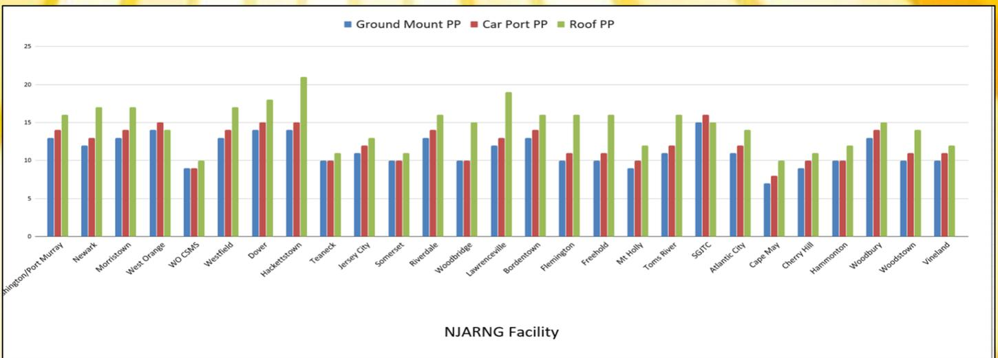
Payback periods for NJARNG facilities for ground-mounted solar panels (blue), car port panels (red), and roof-mounted solar panels (green)
