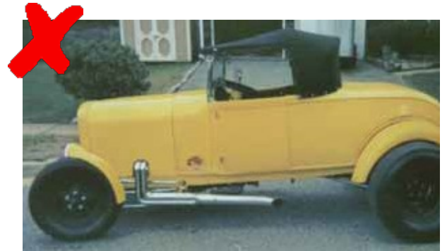
This vehicle does not qualify because it has been altered from its original manufacturer design. The most obvious giveaway is that the vehicle has side pipes. This vehicle is eligible for Street Rod plates.
