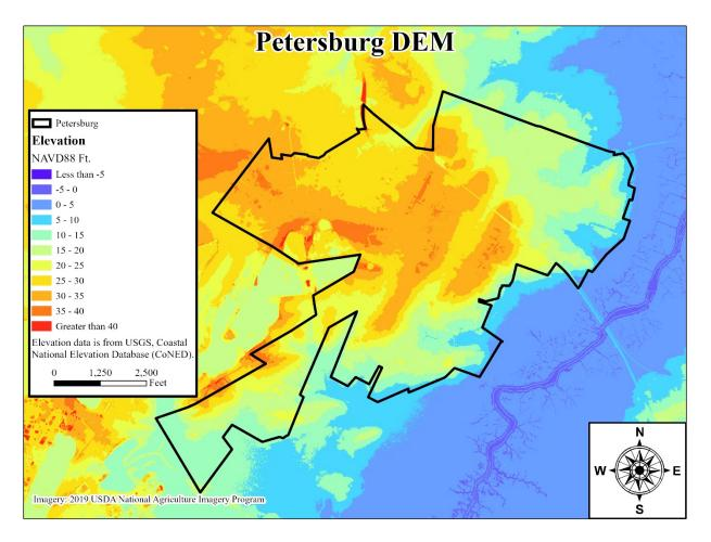
Figure 13. Petersburg Elevation derived from the CoNED DEM. Average land elevations exceed 10.0 feet NAVD 1988.
