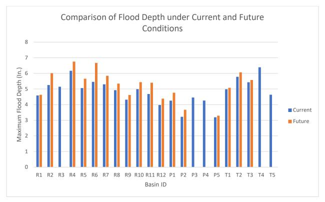
Figure 34. The maximum flood depth for all storm events for both current and future conditions are shown.
