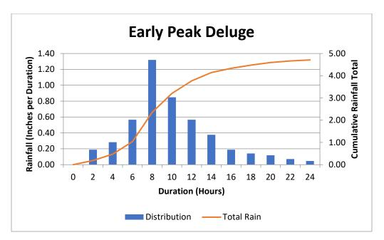
Figure 26. Hyetographs that were used to determine rainfall distributions.
