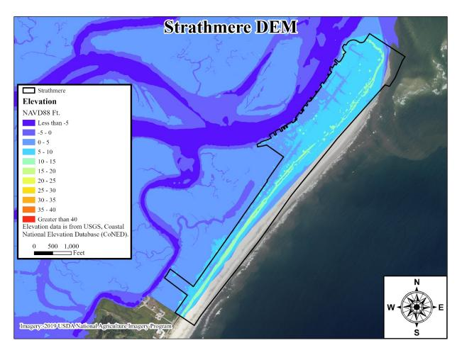
Figure 7. The elevations of Strathmere derived from a DEM. The dune ridge is the main area above 10 feet NAVD 88 in elevation. The development lies between 5 and 10 feet in elevation.
