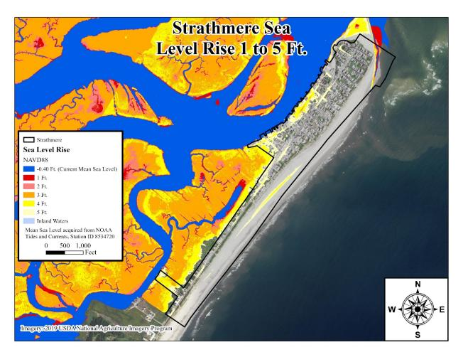
Figure 8. Sea level rise based on 1 foot intervals for Strathmere. Four to five feet of sea level rise invades the developed area.
