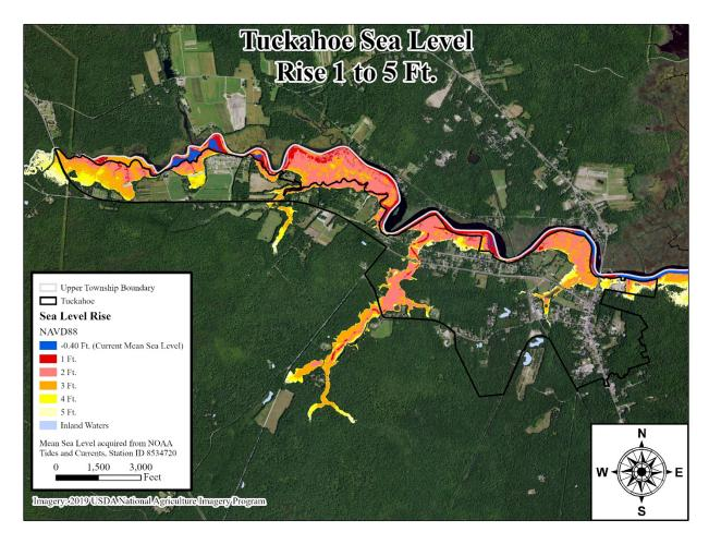
Figure 17. Sea level rise from 1 to 5 ft. for Tuckahoe. Water moves up tributary channels and across the floodplain.
