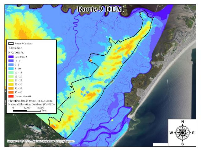
Figure 10. Shows the DEM for the Route 9 Corridor section of Township of Upper. Elevation averages exceed 10.0 feet NAVD 1988.
