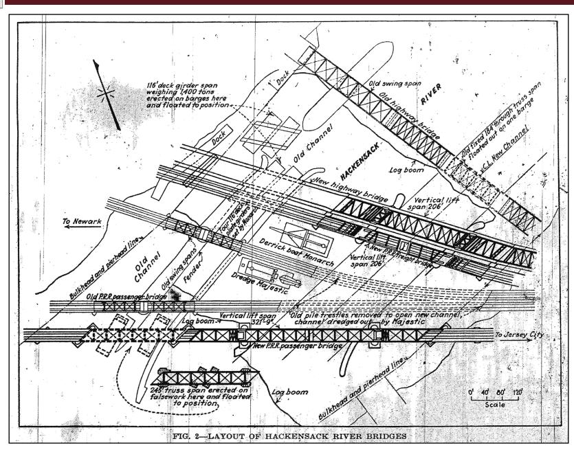
Figure 3: Layout of the Hackensack River Bridges showing the sequence of construction in 1930. (Two Bridge Spans Floated Into Place on Hackensack River, Railway Age, 13 Nov 1930: 778).
