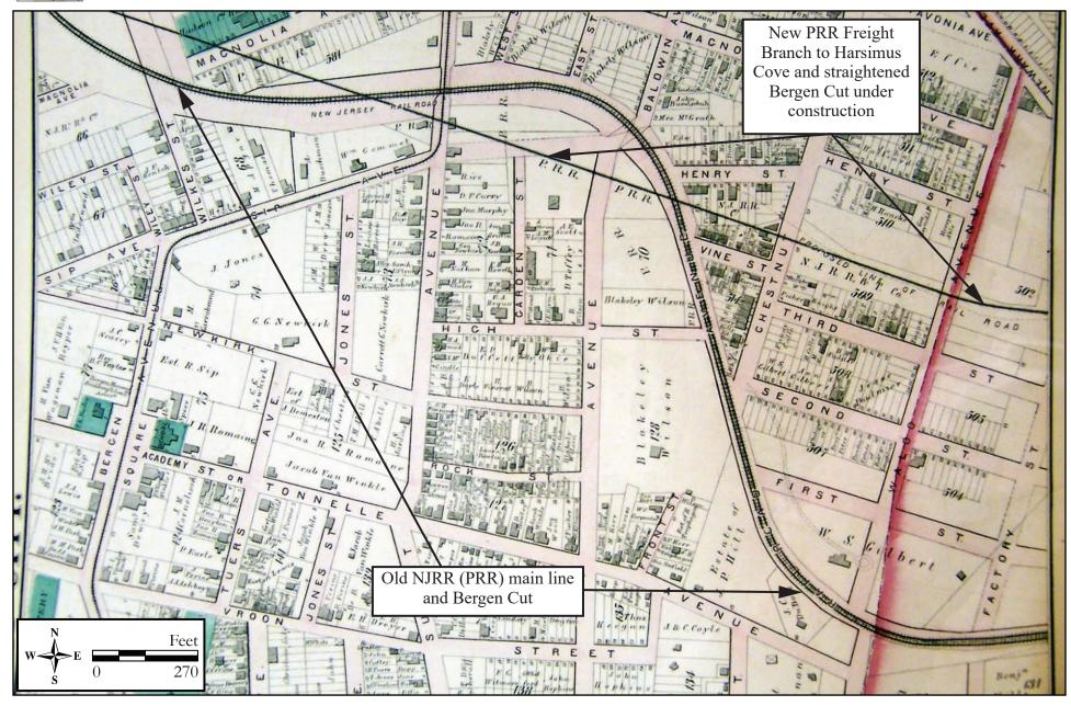
Figure 9: 1878 G.M. Hopkins, Outline and Index Map of Hudson County, New Jersey. Showing a portion of the old New Jersey Railroad alignment of the Bergen Cut and a portion of the new Pennsylvania Railroad straightened alignment.
