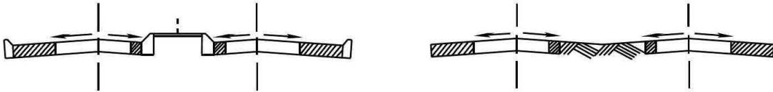
EACH PAVEMENT SLOPES TWO WAYS
