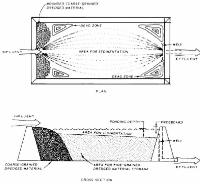
Figure 1- Conceptual diagram of a dredged material containment area
