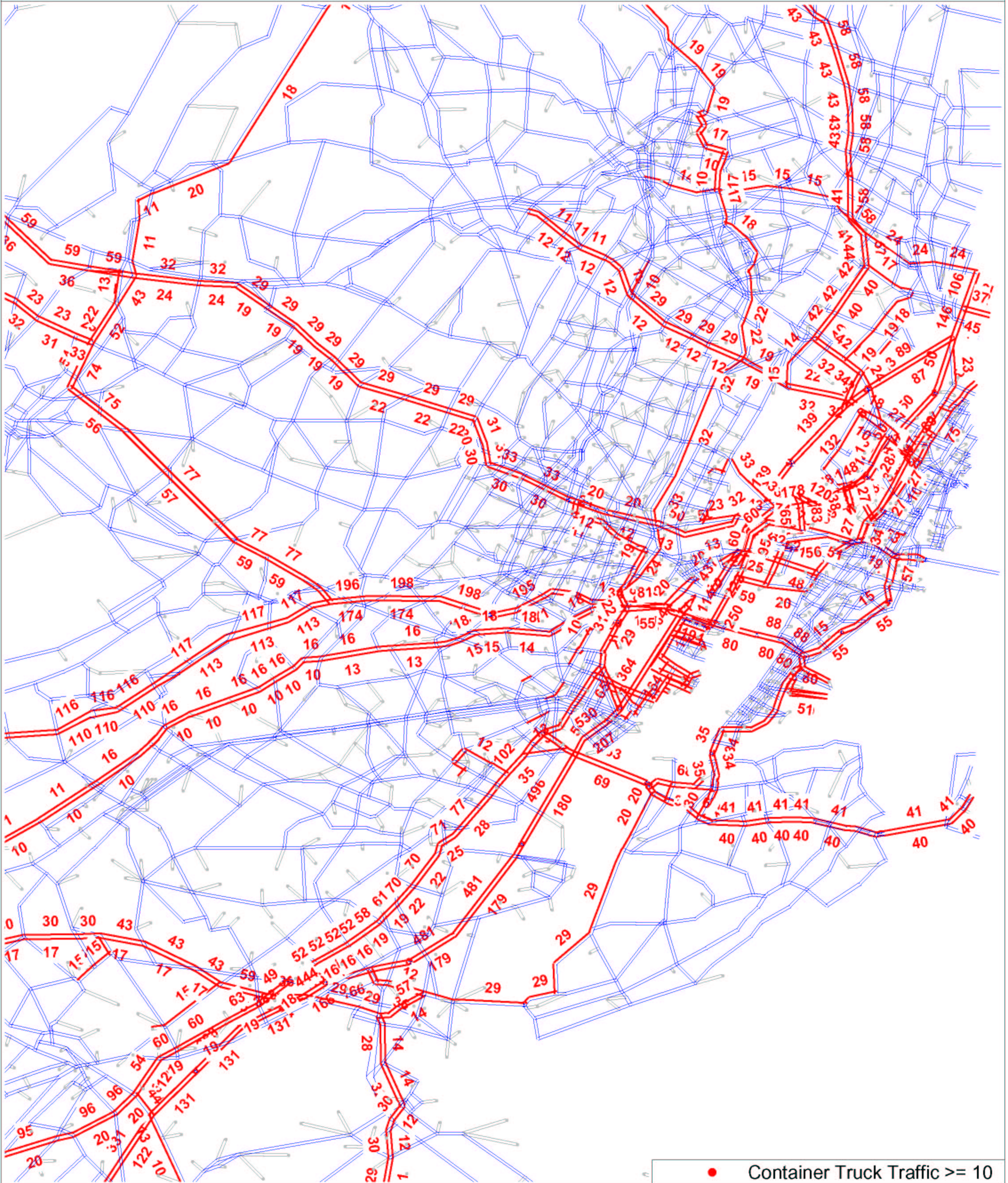
Figure IX.2 Future Container Truck Traffic - PM Peak Hour 2025 NB - High Growth With No PIDN
